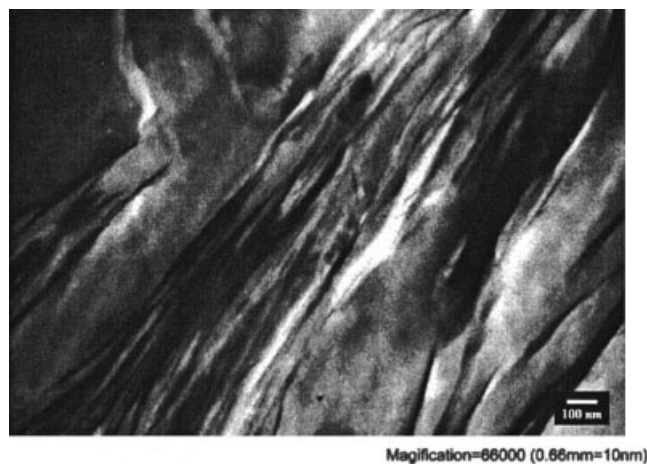
Figure 7 The TEM photograph of polystyrene-montmorillonite nanocomposite [clay contents = 5 wt %].
